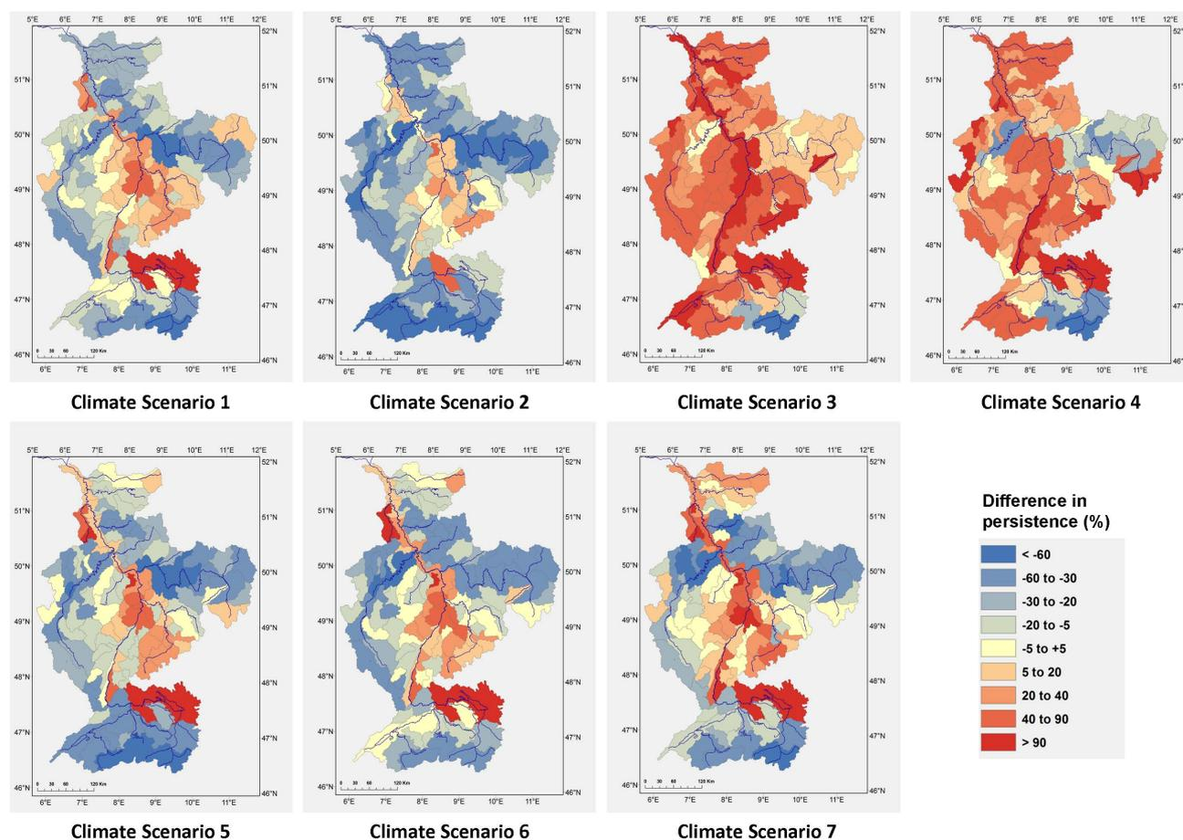
**Fig. 4.** Relative differences (%)<sup>\*</sup> between low flow persistence estimated from simulated low flows using simulated inputs from seven climate scenarios for the reference period 1964–2007 (case 3) and simulated low flows using observed inputs for the same period (case 2). <sup>\*</sup> (Based on simulated input – Based on observed input)/Based on observed input.
