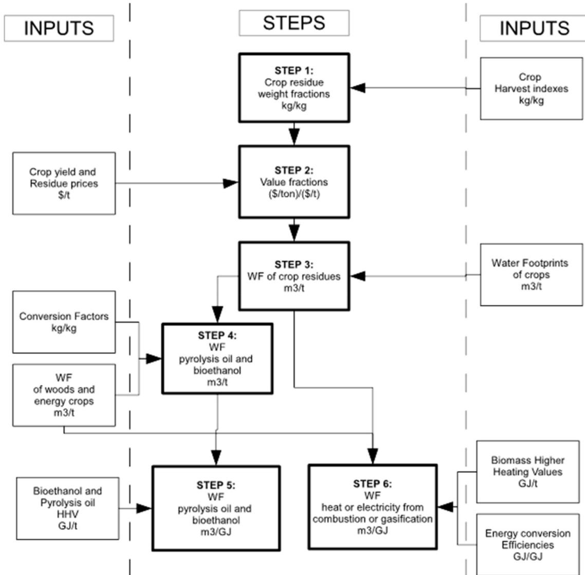
Fig. 1. Six steps for the calculation of the WF of second-generation bioenergy.
