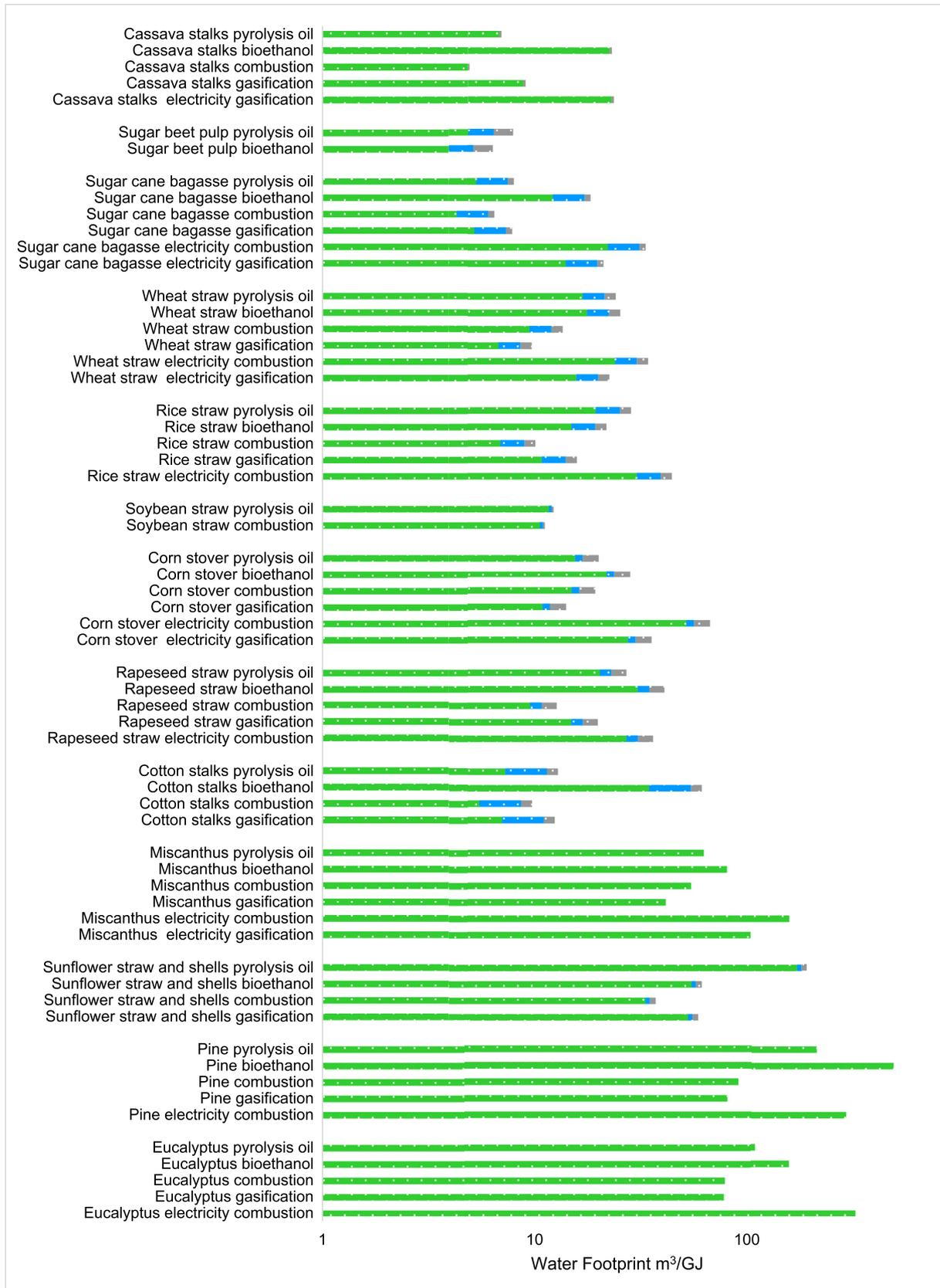
Fig. 7. Green, blue and grey water footprint of pyrolysis oil, bioethanol, heat and electricity from 10 crop residues, 2 types of wood and miscanthus. Logarithmic scale. (For interpretation of the references to colour in this figure legend, the reader is referred to the web version of this article.)
