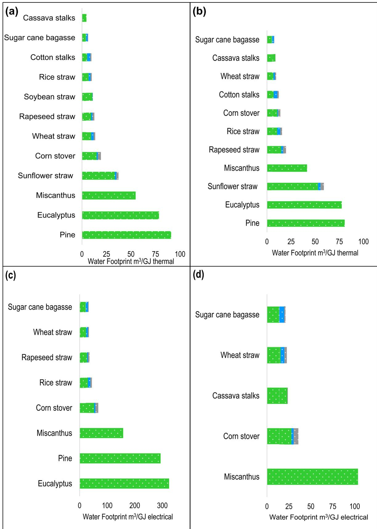
**Fig. 6.** Green, blue and grey water footprints of second-generation bioenergy from crop residues, miscanthus and wood using four different conversion techniques (m³/GJ): (a) combustion, (b) gasification, (c) electricity generation after combustion and (d) electricity generation after gasification. (For interpretation of the references to colour in this figure legend, the reader is referred to the web version of this article.)
