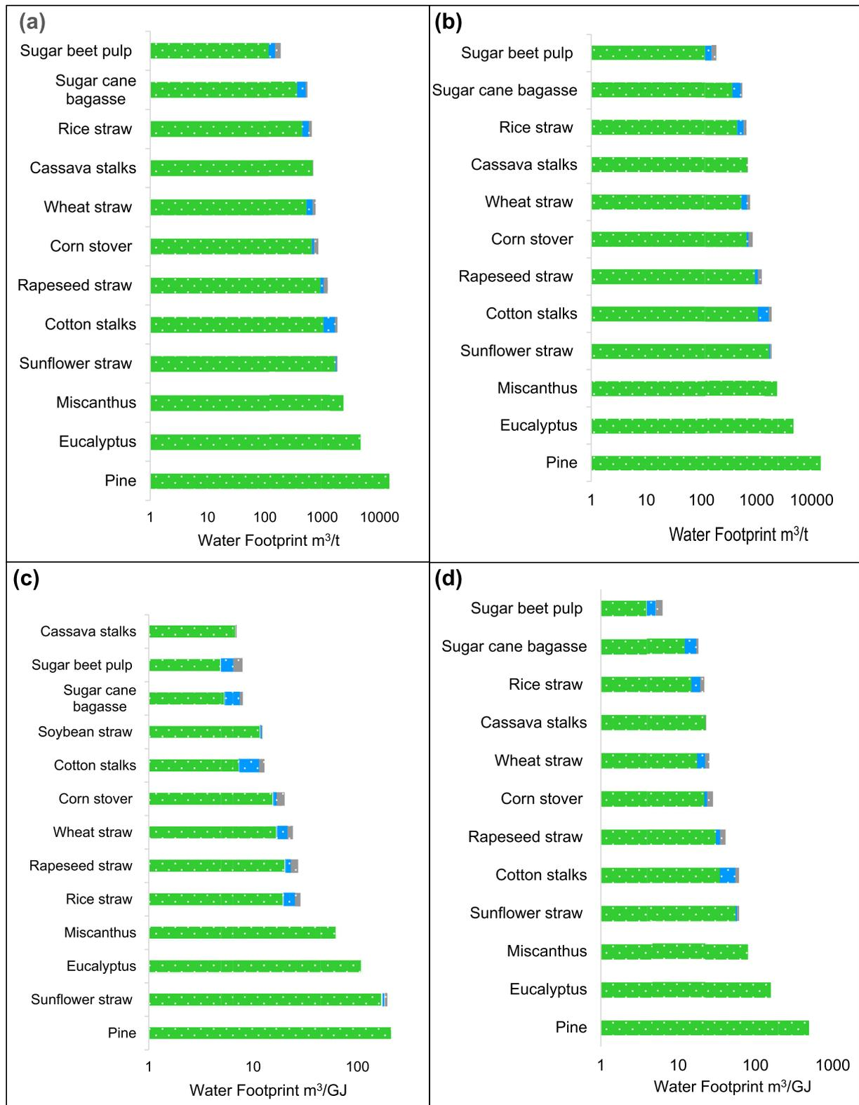
**Fig. 5.** Green, blue and grey water footprint of pyrolysis oil (a,c) and bio-ethanol(b,d) from 10 crop residues, 2 wood types and miscanthus, in m<sup>3</sup>/tonne (a,b) and in m<sup>3</sup>/GJ at logarithmic scale (c,d). (For interpretation of the references to colour in this figure legend, the reader is referred to the web version of this article.)
