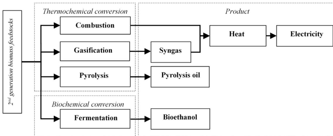
Fig. 2. Thermochemical and biochemical biomass feedstock conversion pathways and the resulting products syngas, pyrolysis oil, bioethanol, heat and electricity.
